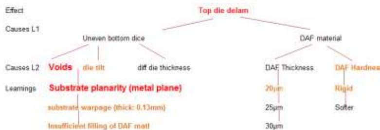
Fig. 5. Fault-tree analysis
